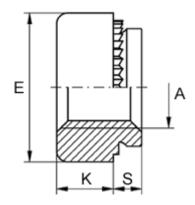
Female thread A = M2Height K = 2.0 Max recess height = 1.0 Min distance to edge = 3.0Outer diameter E = 6.0
